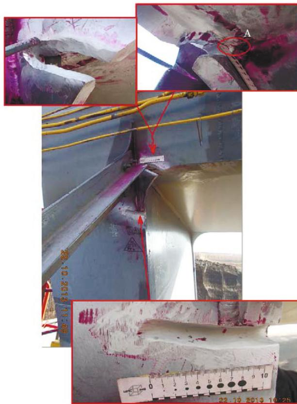
Fig. 8. Grinded fillet weld at the left column of the P frame (detail A at Fig. 10).
