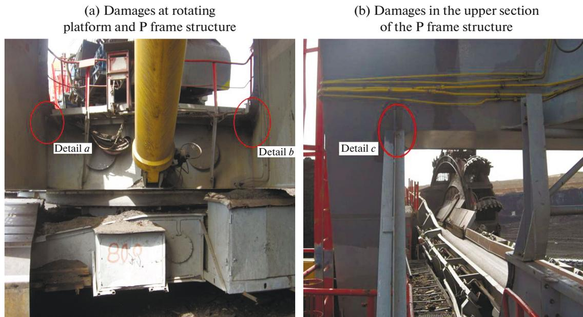
**Fig. 2.** Damages at the vital structure of the bucket-wheel boom.
