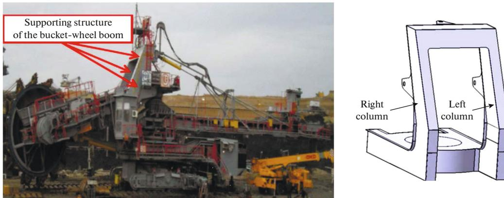
**Fig. 1.** Bucket-wheel excavator SchRs 800 in the open pit mine “Kostolac”—Serbia and model of the vital structure of the bucket-wheel boom (rotating platform and P frame).
