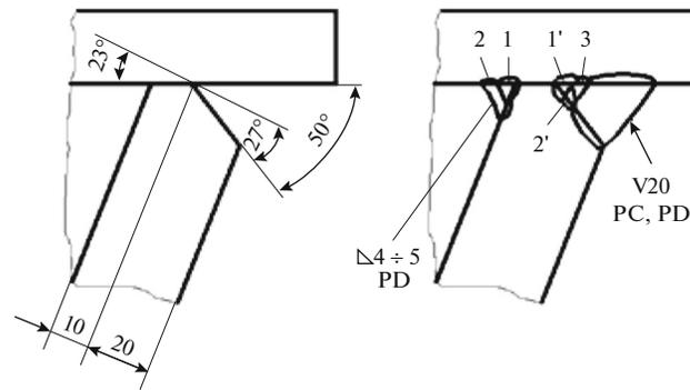
Fig. 12. Preparation for welding and sequence of passes—fillet welded joints at the support structure of the bucket-wheel boom.
