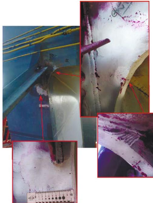
**Fig. 17.** Examined repair welded joint at the right side of the structure of the rotating platform.
