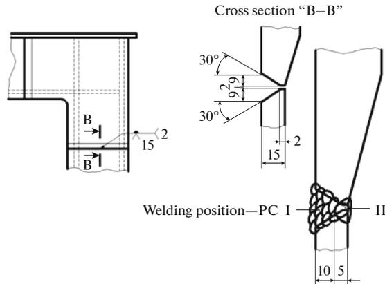
**Fig. 14.** Preparation for welding – butt welded joints at the structure of the P frame left column.
