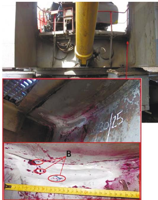
**Fig. 10.** Grinded section at the left side of the rotating platform.
