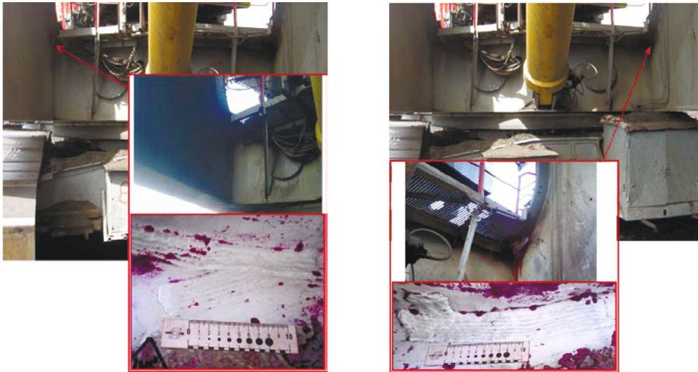
**Fig. 5.** Damages at parent material of the rotating platform and welded joints detected during penetrant testing.
