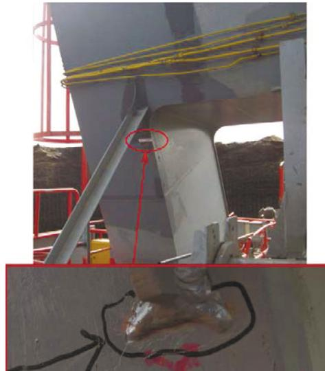
**Fig. 4.** Crack on the surface of fillet welded joints, left side of the column—detail c (crack length  $L = 40$  mm).
