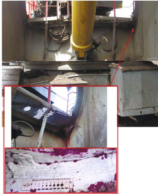
Fig. 18. Examined repair welded joint at the left side of the structure of the rotating platform.
