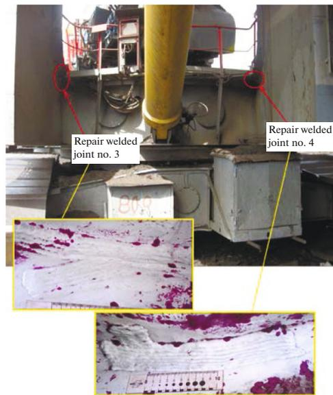
**Fig. 16.** Examined repair welded joint at the structure of the rotating platform, internally designated with nos. 3 and 4.
