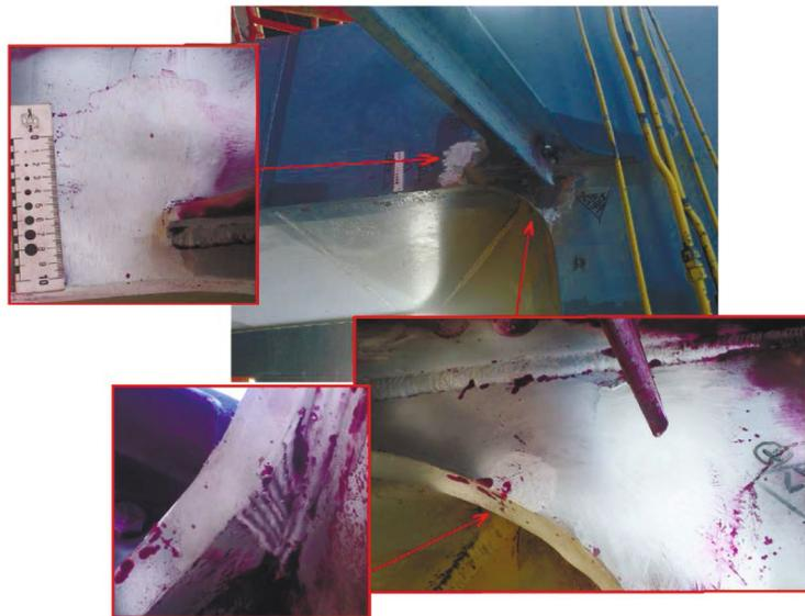
**Fig. 6.** Damages at parent material of the P frame and welded joints detected during penetrant testing (left side—Fig. 3, detail *c*).
